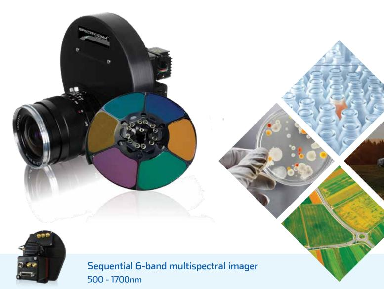
SpectroCam Short Wave InfraRed (SWIR) multispectral cameras deliver sequential full-frame images for up to 6 spectral bands between 500 – 1700nm at rates up to 30 frames per second (~5 stacks per second). Using standard and custom interchangeable filters, SpectroCam images the spectral bands fit to your specific applications. These cameras incorporate a high-sensitivity solid state InGaAs sensor, available in SWIR (1000 – 1700nm) and VIS-SWIR (500 - 1700nm)
